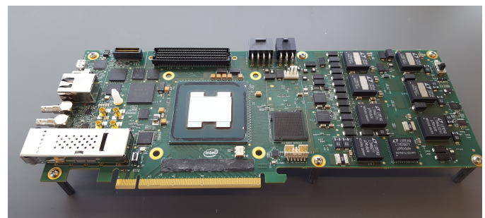
Fig. 14: Delidded Stratix 10 FPGA on development board
